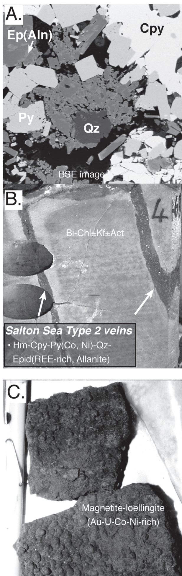
Figure 8: Fe-oxide-rich mineral assemblages in veins and scales from the Salton Sea geothermal system, California.
