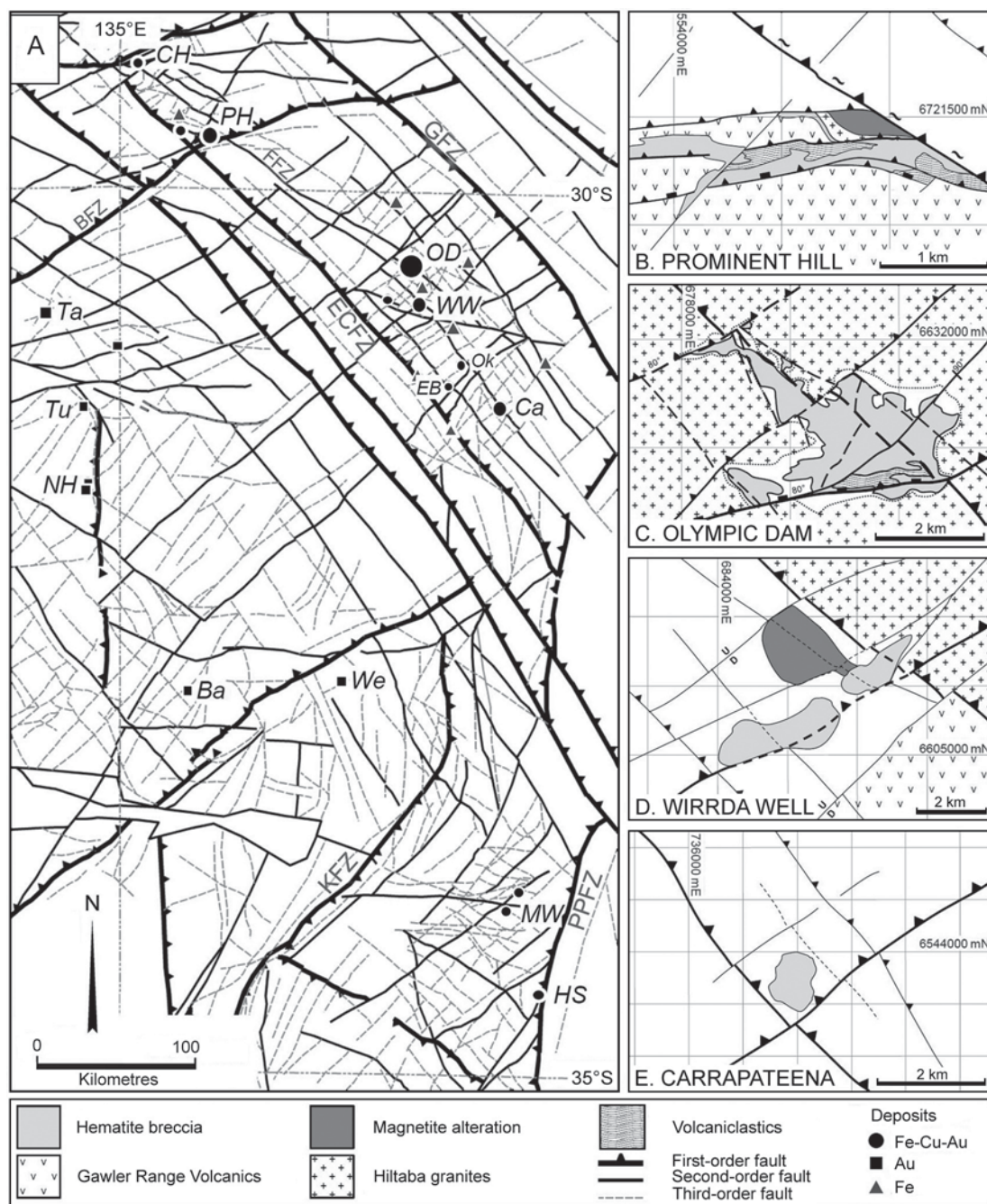
Figure 8: (A) Basement structural geology interpretation for the Olympic IOCG Province with IOCG, gold and iron deposits and prospects. Insets show deposit-scale basement structural geology interpretations for Prominent Hill (B), Olympic Dam (C), Wirrda Well (D) and Carrapateena (E) based on aeromagnetic and gravity imagery. Prominent Hill geology modified after Belperio et al. (2007). Olympic Dam geology modified after Widdup et al. (2004). Unpatterned areas in insets represent older (pre-Hiltaba) rock units. Deposit labels as per Fig. 5. Fault labels as per Fig. 1, including BFZ – Bulgunnia Fault and FFZ – Fitzgerald Fault.
