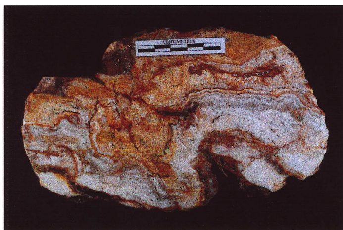
Photograph 11 : Colloform banded epithermal vein quartz, Kyaukmyet.
