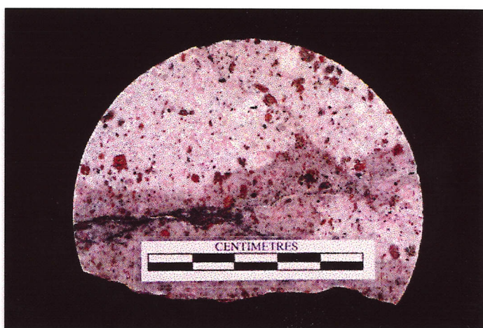
Photograph 6 : Dacite porphyry with feldspar phenocrysts replaced by crystalline pink alunite, dickite and chalcocite, Letpadaung deposit.
