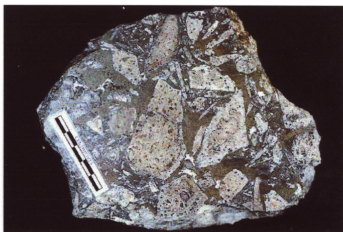
Photograph 4 : Pyrite-chalcocite breccia matrix hosted mineralisation, Sabedaung open pit.
