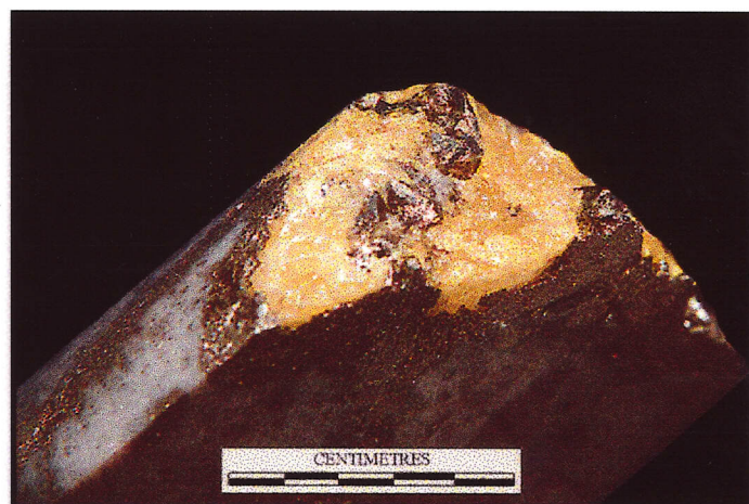
Photograph 10 : Silicified brecciated dacite porphyry with matrix native sulphur and crystalline chalcocite, Letpadaung deposit.
