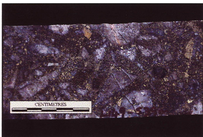
Photograph 5 : Mineralised hydrothermal breccia with matrix pyrite-chalcocite. DDHL149-539 m, Letpadaung deposit.
