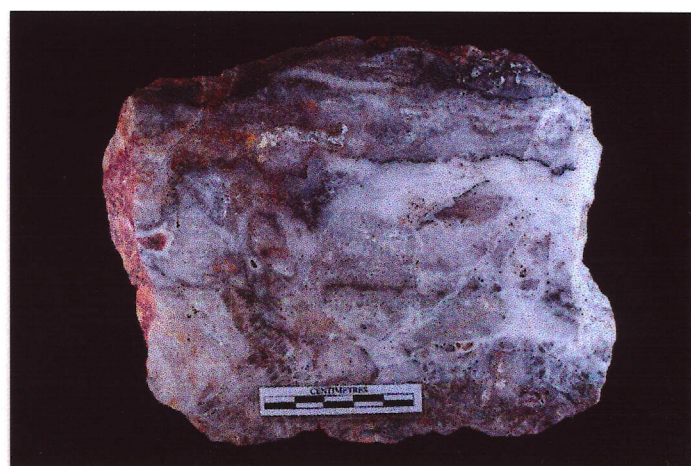
Photograph 12 : Multiphase epithermal quartz vein breccia, Kyaukmyet.
