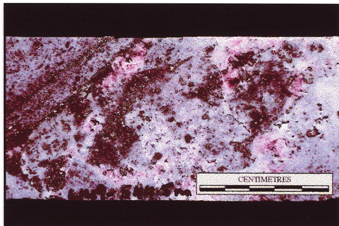
Photograph 8 : Silicified dacite porphyry breccia with matrix bladed pink alunite, Letpadaung deposit.
